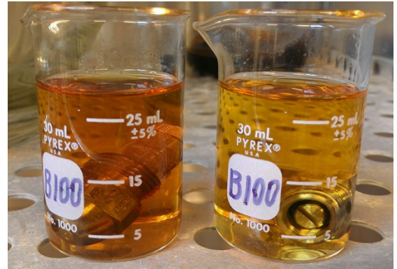
Figure 5 Fuel nozzles exposed to B20 blends for 4 weeks at 175 F. Left - brass nozzle, Right - stainless steel nozzle.
