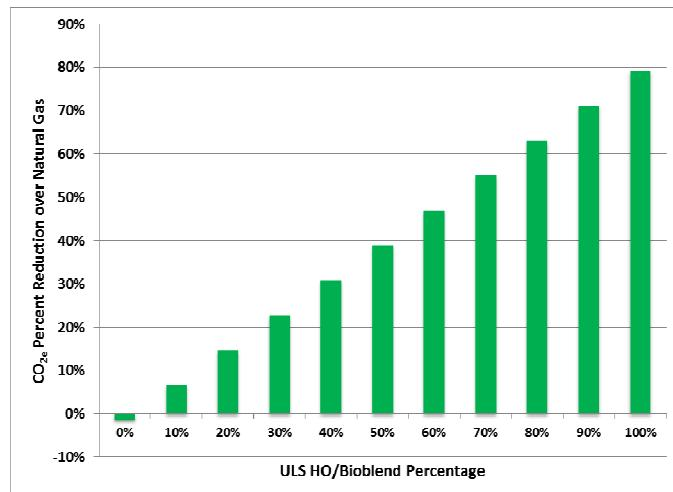
**Figure 5** shows that, as technology advances, biodiesel blends with heating oil, CO<sub>2e</sub> reduction can far exceed conventional natural gas and shale gas. Given that biodiesel blends with heating oil GHG emissions can easily be lower than natural gas GHG emissions, there is no climate change reason for fuel switching from oil to natural gas.
