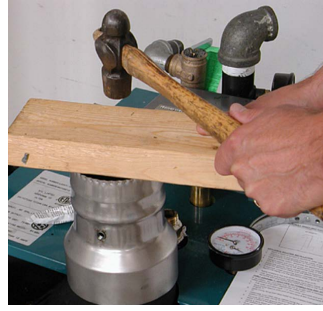
15. Drive the adapter onto the appliance using a mallet and block of wood.
