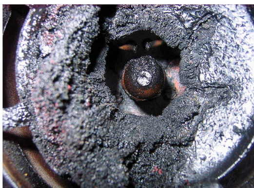
Figure 5: Coking of oilburner nozzle.
