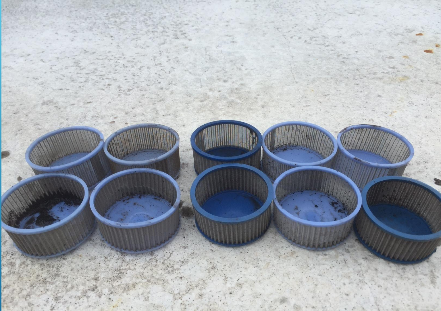
STRAINERS RECOVERED FROM ROUTINE SERVICE @ BRIDGEPORT CT
