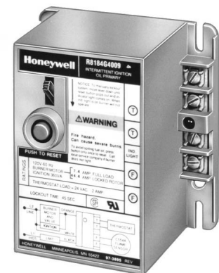
⚠ Power Supply, Provide Disconnect Means and Overload Protection as Required ⚠ To Use R8184 with Line Voltage Controller, Jumper T-T Terminals and Connect Line Voltage Thermostat in Series with Limit Controller.
