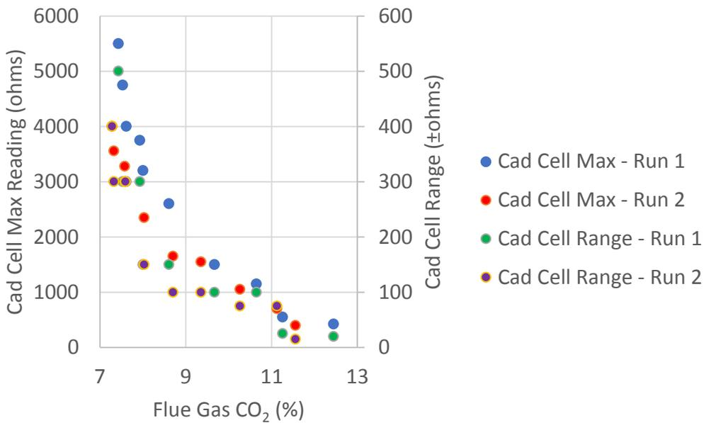
Figure 15 B100 Tallow Cad cell max reading and range
