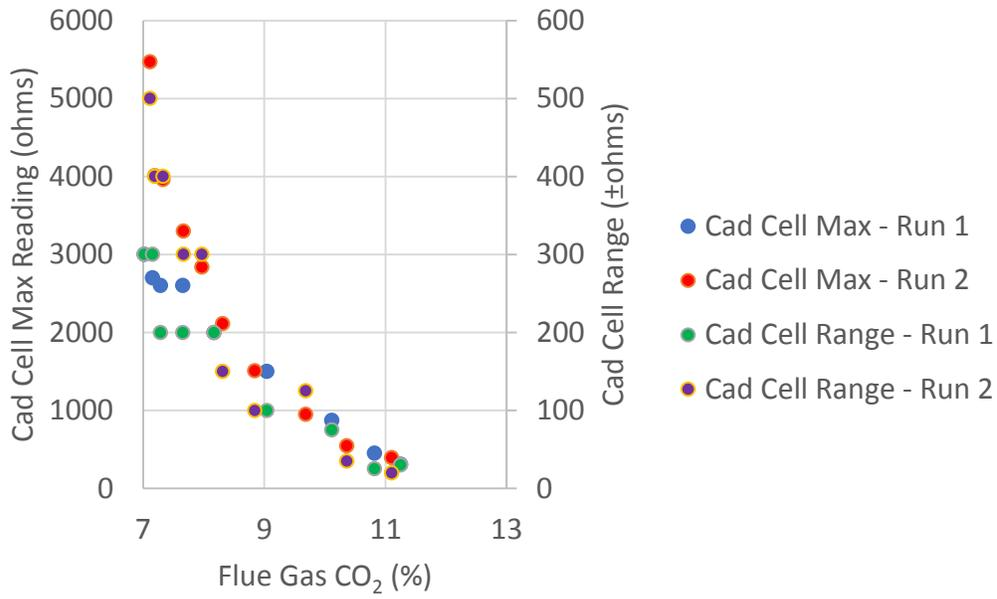
Figure 12 B100 Soy Cad cell max reading and range
