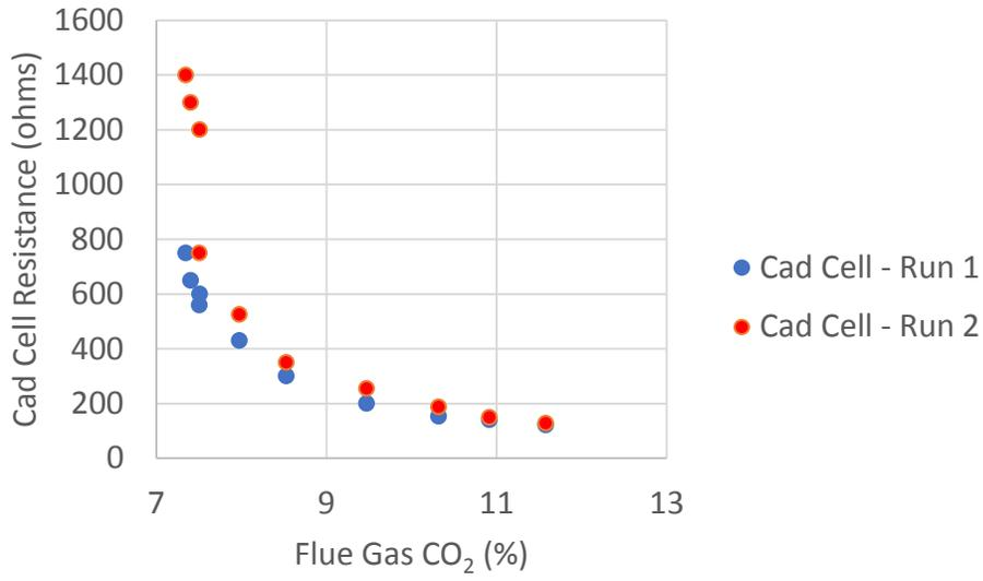
Figure 2 B0 Average cad cell resistance
