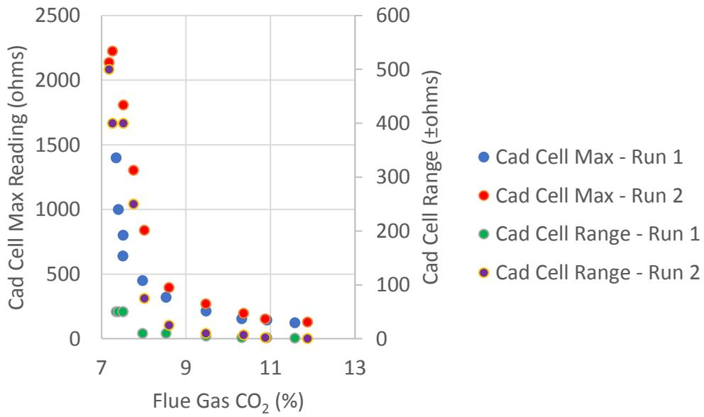
Figure 3 B0 Cad cell max reading and range
