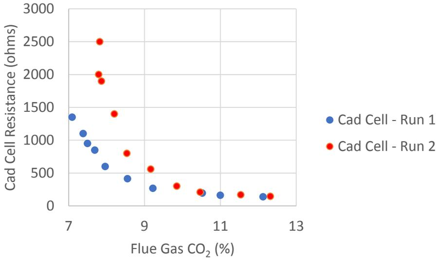
Figure 5 B20 Soy Average cad cell resistance
