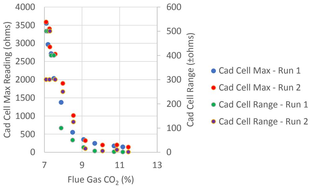
Figure 9 B20 Tallow Cad cell max reading and range
