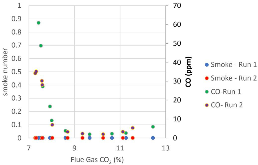
Figure 13 B100 Tallow Flue gas smoke number and CO
