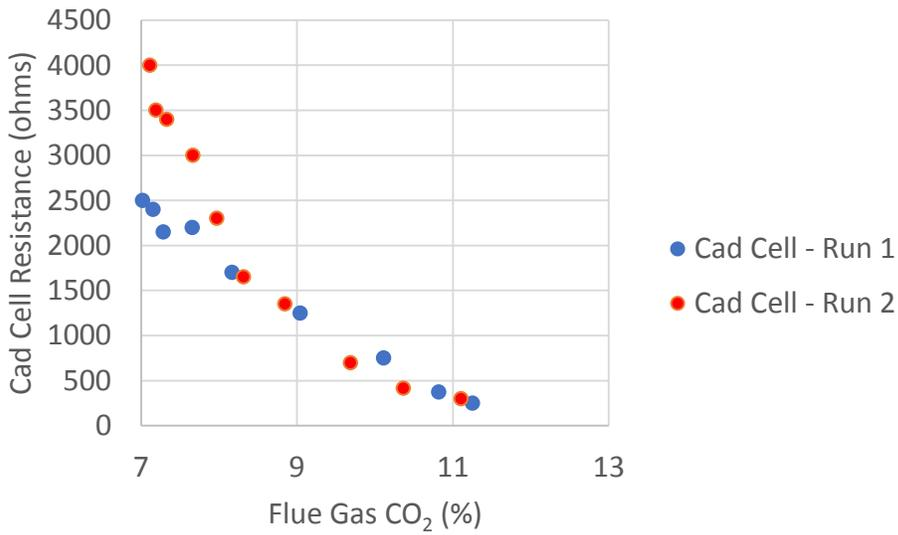
Figure 11 B100 Soy Average cad cell resistance
