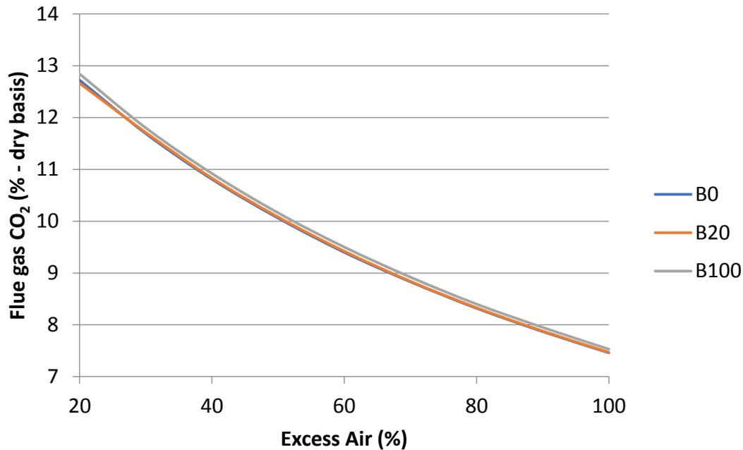
*Figure 16 Relationship between flue gas CO<sub>2</sub> and excess air for different fuels.*
