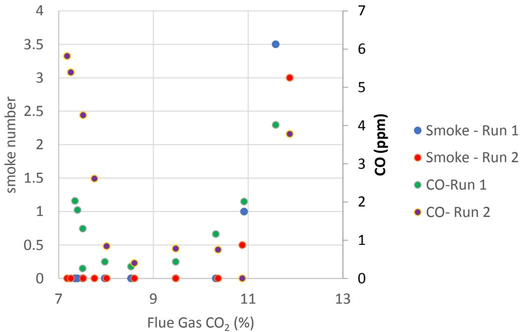
Figure 1 B0 Flue gas smoke number and CO
