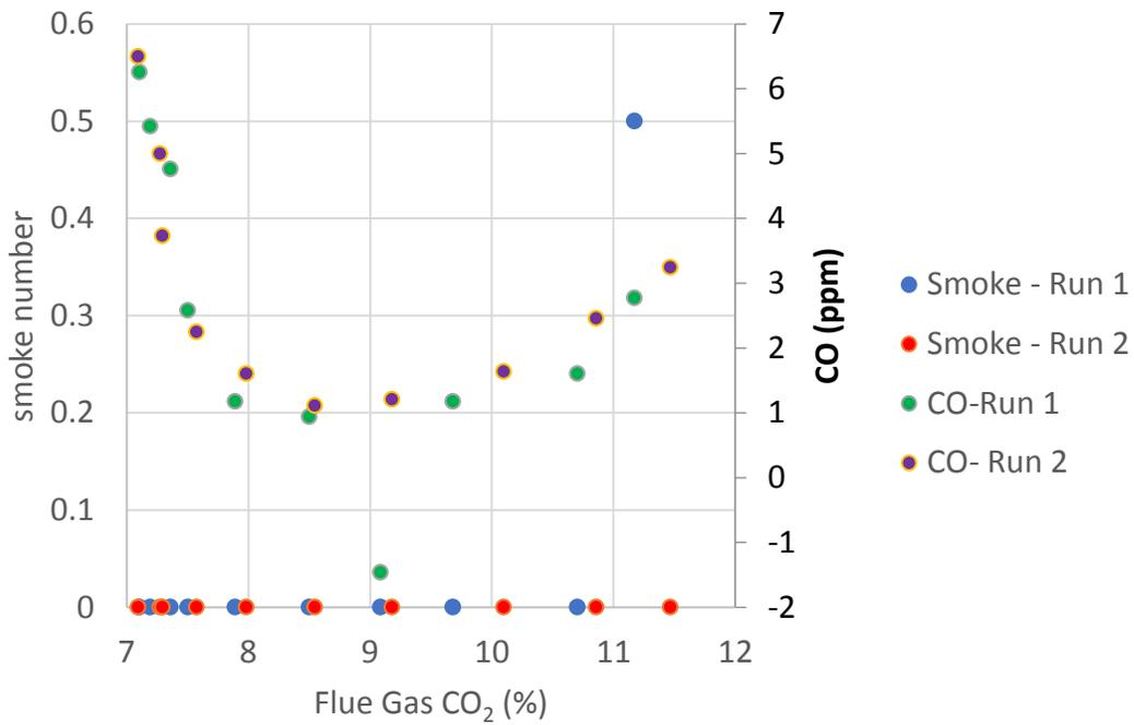
Figure 7 B20 Tallow Flue gas smoke number and CO
