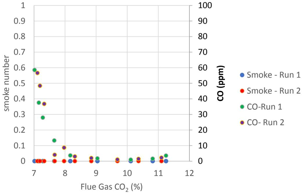
Figure 10 B100 Soy Flue gas smoke number and CO
