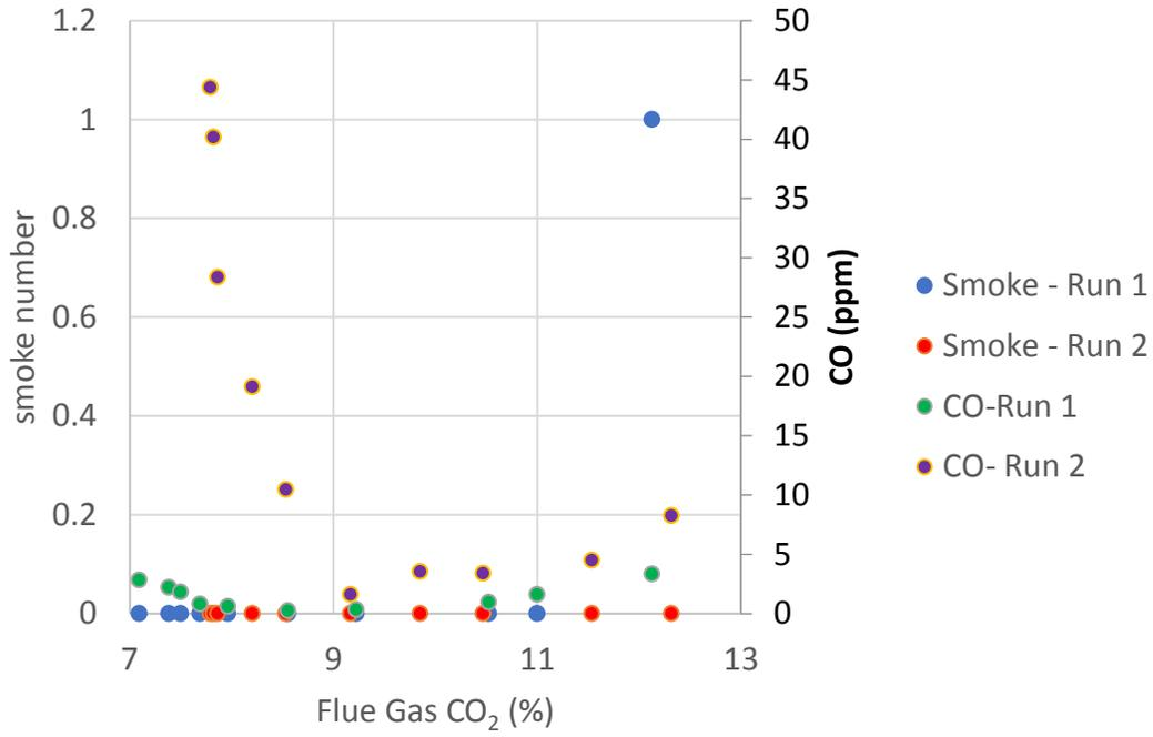
Figure 4 B20 Soy Flue gas smoke number and CO
