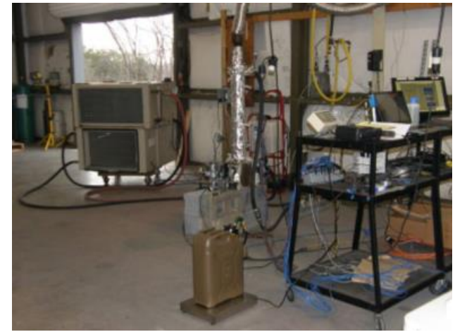
Horizontal burner proof test with desorber
