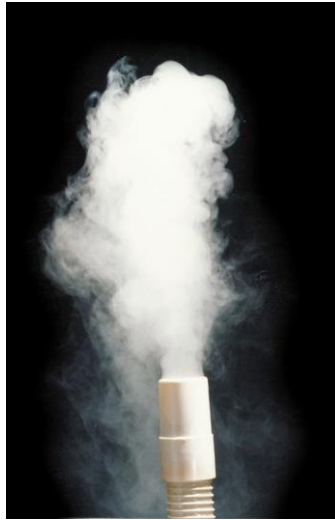
Uniformed Dispersion of Fine Liquid-Fuel Particles
