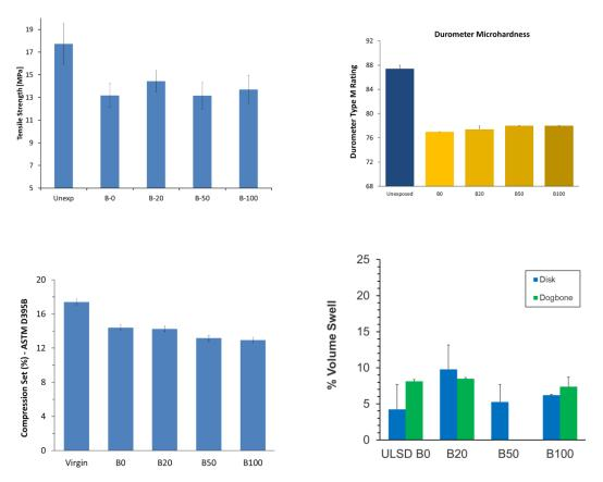
To confirm performance in actual operation, pumps representing the vast majority of those installed in the U.S. were run for 7000 hours using a 5 minute on / 1 minute off control cycle pattern with 12% (B12) and 20% (B20) biodiesel blended with both high and ultra-low sulfur conventional petroleum-based No. 2 heating oil. Seven (7) pumps were run using each fuel, and
