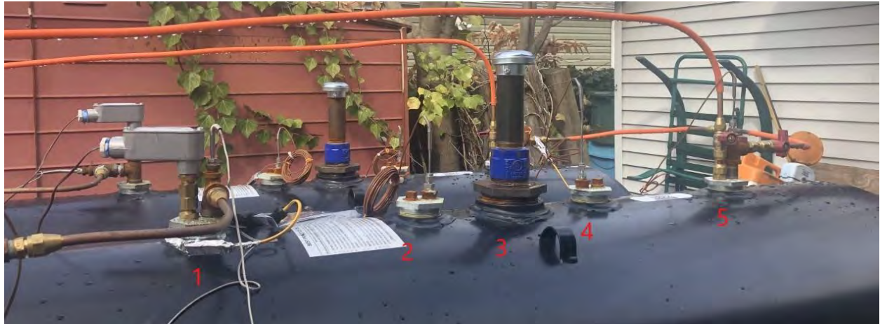
Figure 2: Field picture of steel tank used in the study with the various bungs labeled
