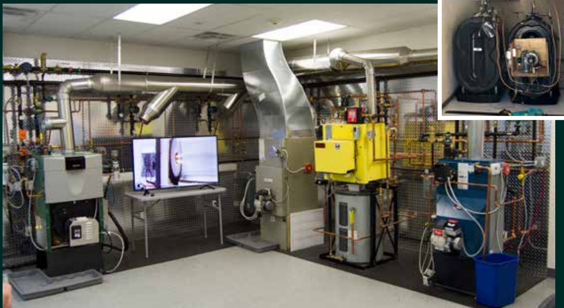
NORA Liquid Fuels Laboratory, Plainview, NY (inset, NORA Freezer for testing fuel cold flow properties)
