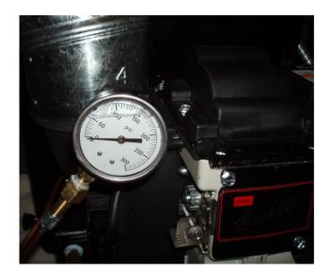
1 - Attach pressure gauge to end of copper connector tube
