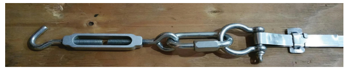
Fig. 12. CR metal band & Clamp with D ring and turnbuckle
