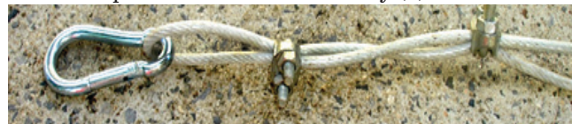
Fig. 11. CR metal wire rope with u-clamps and quick link
