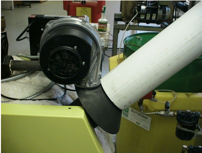
Figure 20 Annular eductor mounted on prototype, high efficiency Energy Kinetics boiler
