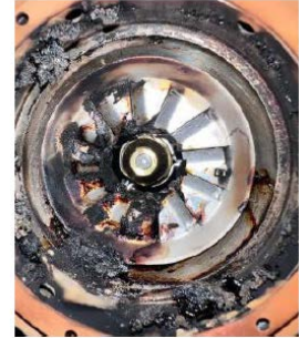
Figure B-5. Example of retention head with a rating of 4
