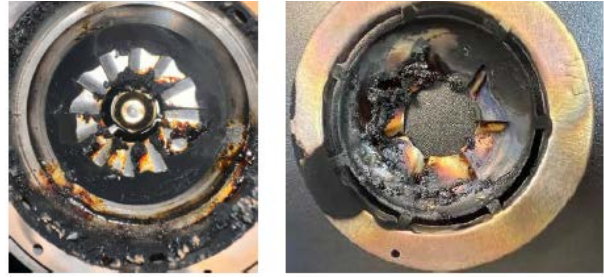
Figure B-4. Examples of retention heads with a rating of 3
