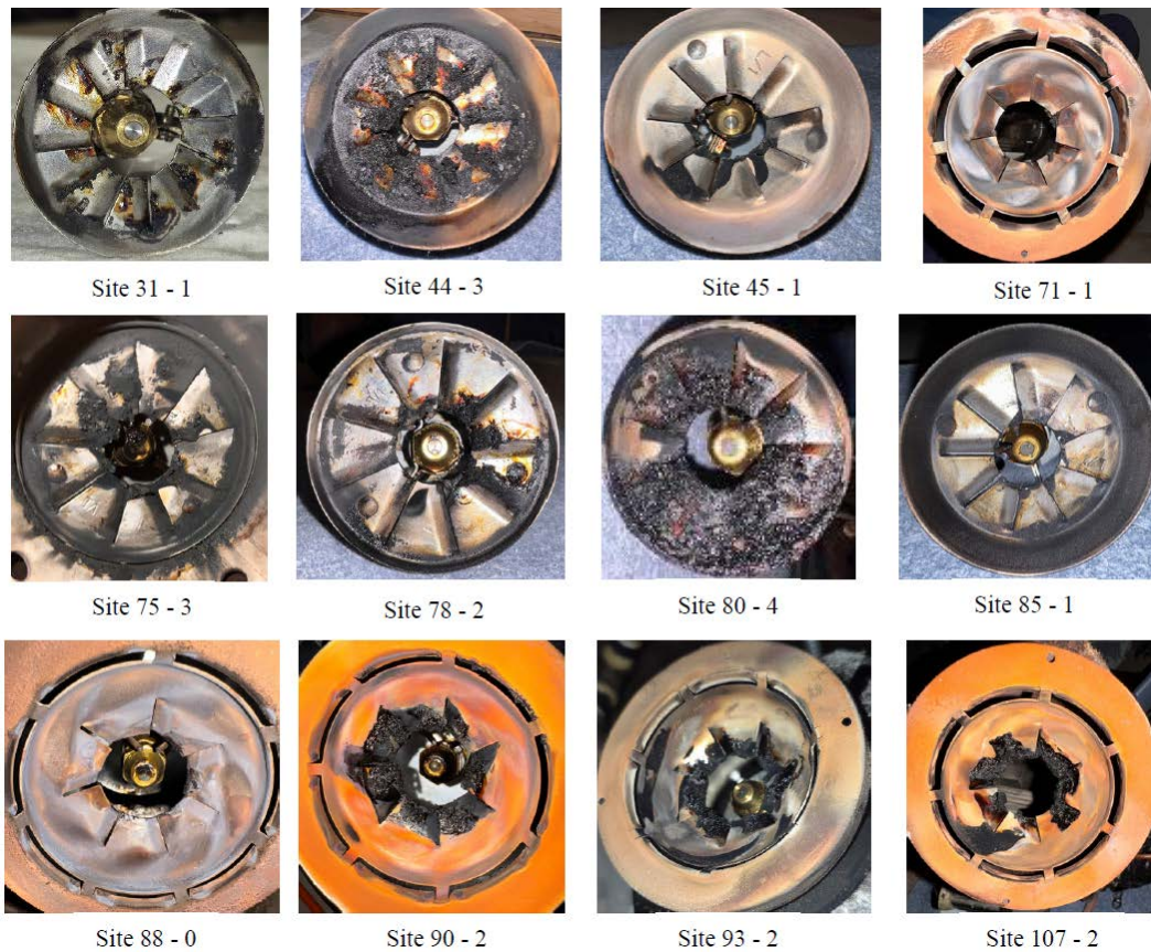
Figure 5. Photos of the retention heads from select Level 2 sites with hot chamber boilers during visit period 5. The number after the dash indicates the coking level score.
