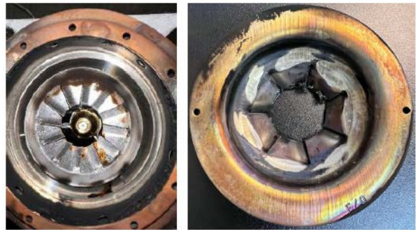
Figure B-1. Examples of retention heads with a rating of 0
