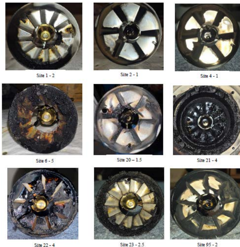
Figure 6. Photos of the retention heads from all sites with cold chamber boilers during visit period 5. The number after the dash indicates the coking level score.
